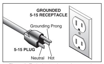
Figure 2. Typical 5-15 plug and receptacle.
